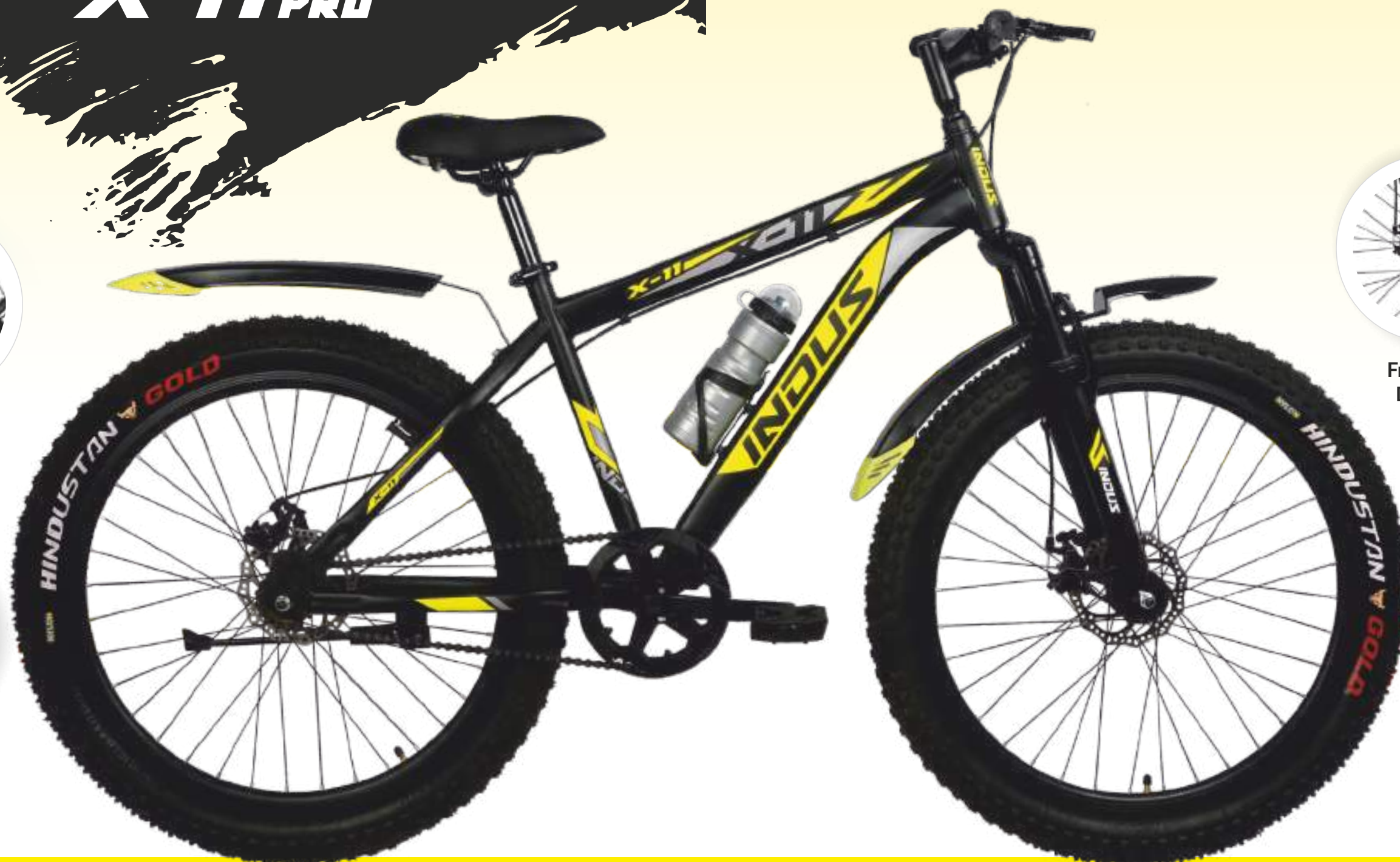
38.10 mm Heavy Duty Suspension Fork for Off Road
